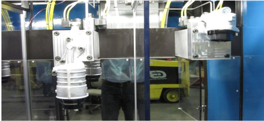
Test filter adapters are available for most filter housing types Multiple filter types can be tested simultaneously
